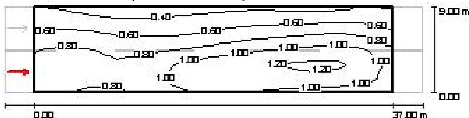
Figura 5.3 – luminanza a terra – curve isolux.
