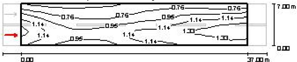
Figura 5.1 – luminanza a terra – curve isolux.
