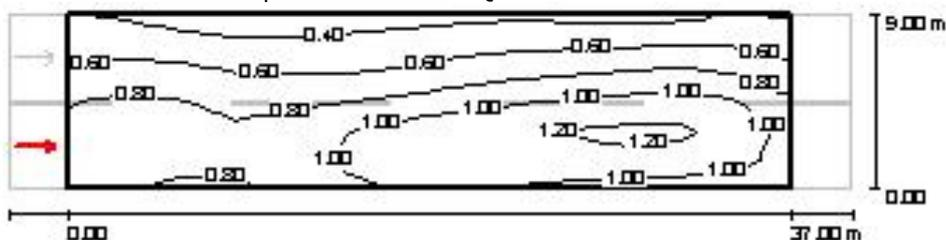
Figura 5.5 – luminanza a terra – curve isolux.
